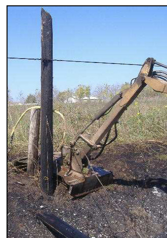
DANGEROUS SITUATION... (Above) The arm of the mower which cut the power pole, causing the line to fall down onto the tractor and catch fire. (Left photo) The remains of the burned-up transformer pole.
